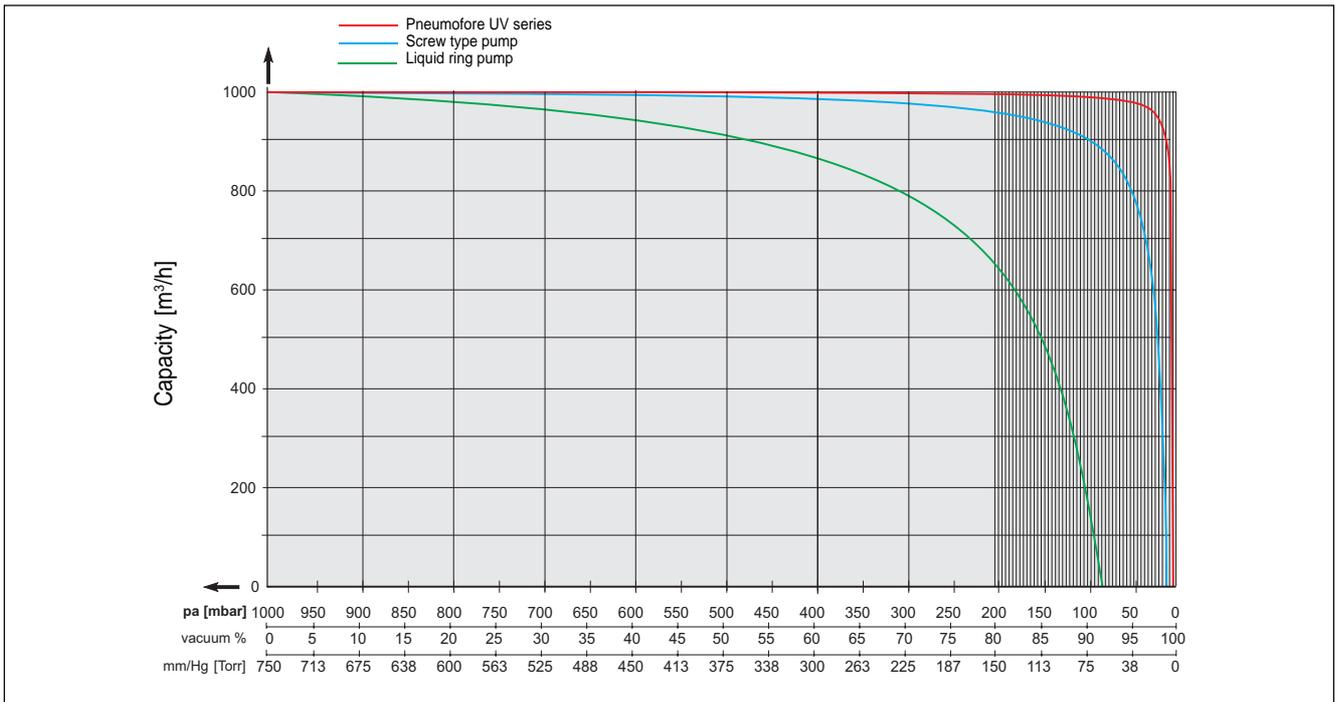
Fig. 3 - Data on capacity of vacuum pumps with changes in vacuum degree (absolute pressure)
